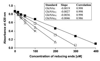
Fig. 1. Calibration of the Schales' procedure. The figure shows absorbance at 420 nm versus molar concentrations of GlcNAc ( $\blacksquare$ ), GlcNAc<sub>2</sub> ( $\square$ ), GlcNAc<sub>4</sub> ( $\triangle$ ) and GlcNAc<sub>6</sub> ( $\times$ ) in the 450  $\mu$ l samples. The experiment was carried out in duplicate and the values represent the average. The insert shows the data for the regression lines.
