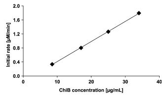
Fig. 5. Initial rates (reducing ends produced per minute) versus ChiB concentration. Data were collected by conducting the experiment depicted in Fig. 4 with various ChiB concentrations. Initial rates were determined by linear regression, using measurements collected before the concentration of reducing ends reached 30  $\mu$ M.
